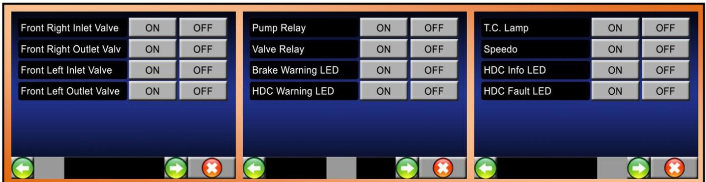
Finally, the utility section provides the user the facilities to perform power brake bleeding, modulator bleeding and a set of four separated corner tests, to test each individual corners ABS assemblies.
